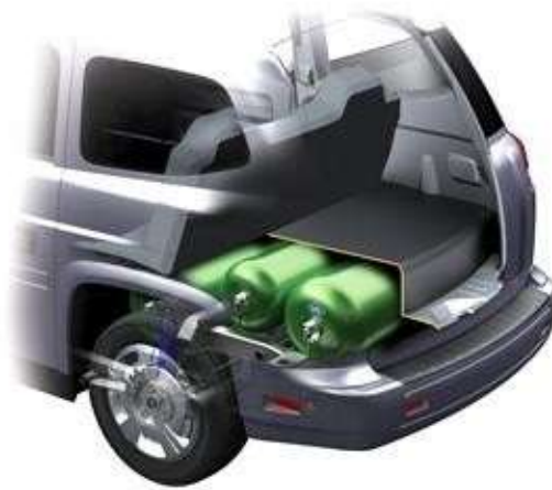
Storage tank of natural gas vehicle [44]
